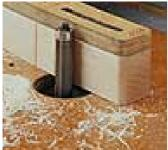
Few things in woodworking are as frustrating as trying to make several irregular-shaped pieces exactly the same. The solution is to use a template and a flush trim bit. The bearing on the bit rides against the edge of the template and trims the work piece to the exact shape of the template.
