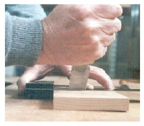
Instead of a marking knife, some old hands use a very short sideways-tilted 25mm (one-inch) chisel with the bevel against the square.
