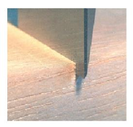
There's only one place to put your chisel when working to a cut line.
