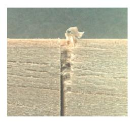
The very first stroke of a tenon saw.
