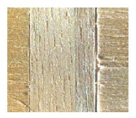
The two sides of the same cross-halvng joint, also in Jelutong. (Two prints were necessary at this magnification, hence the slight difference in colour). Although the joint was a perfect fit, this is not apparent when you look at its right-hand side. Each knife line was struck with the try square and knife position as above. This meant that the crushed side of the left-hand line was in the waste.
