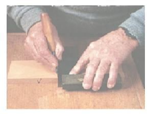
Try grinding a wide bevel on the left-hand side of a fairly thick blade and hold the knife sloping outwards but with the bevel vertical. The wrist should now be in a more natural position, offering greater control.
